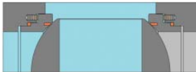
Bi-directional seat Downstream sealing
